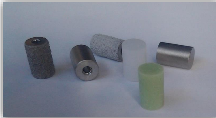
Figure 5: Cylindrical samples of biomaterials commonly used in orthopedic surgery. Left-right: Porous coated titanium, cobalt-chrome, hydroxyapatite covered titanium, polyethylene, polymethyl-metacrylate, and stainless steel (extract from Study II )
